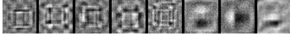
Figure 7. Eight feature detectors of an MLP trained to remove a square blur. The MLP was trained on the blurry patches themselves ( i.e. no pre-processing). The features are large compared to the output patches because the information in the input is very spread out, due to the blur.
